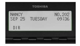
IP5000 4-line LCD display in Idle Mode
