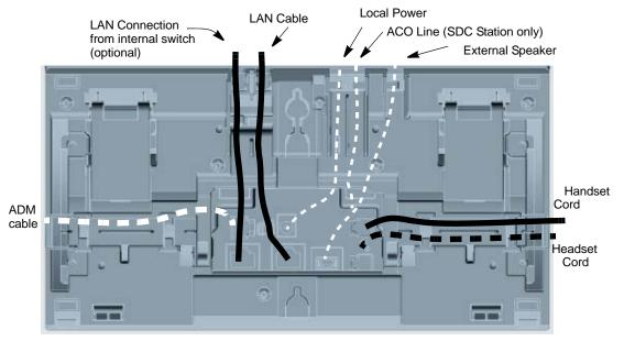
The IP5000-series telephones include the special long-tail handset cords required to fit the tilt bases.
