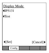
The IP5131 setting allows default operation of the display as it was designed to support 10 LCD keystrips plus 4 lines of call processing/softkey information.
